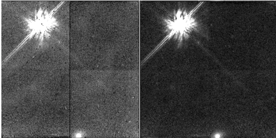
Figure 6. A: OTFR/CALNICA pipeline reduction with synthetic dark and library flats, B: CALNICA with custom-matched dark and linear-regime flat-field.
