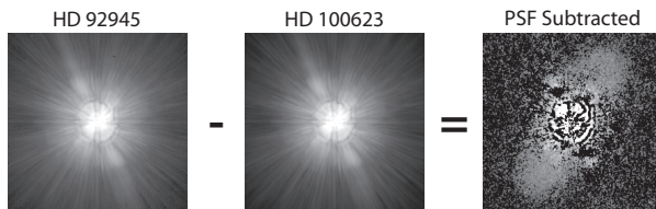
Figure j2. (Left) ACS coronagraph observation of HD 92945 in filter F606W using the r=0.9'' occulting spot. The center of the spot is filled with light due to the aberrated HST optics. The streak running from the upper left to lower right is instrumental scattered light. (Middle) Observation of HD 100623 used as a reference PSF. (Right) Subtraction from HD 100623 from HD 92945. Residuals caused by mismatches between the two images are evident. All images are logarithmically scaled.
