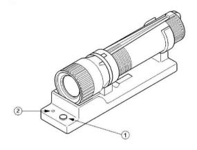
(1) <u>Push-to-Test Button</u> Pressing this button indicates the battery status.
